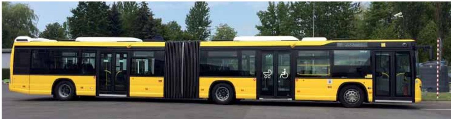
Scania CityWide with the Aerosphere World air conditioning system.
