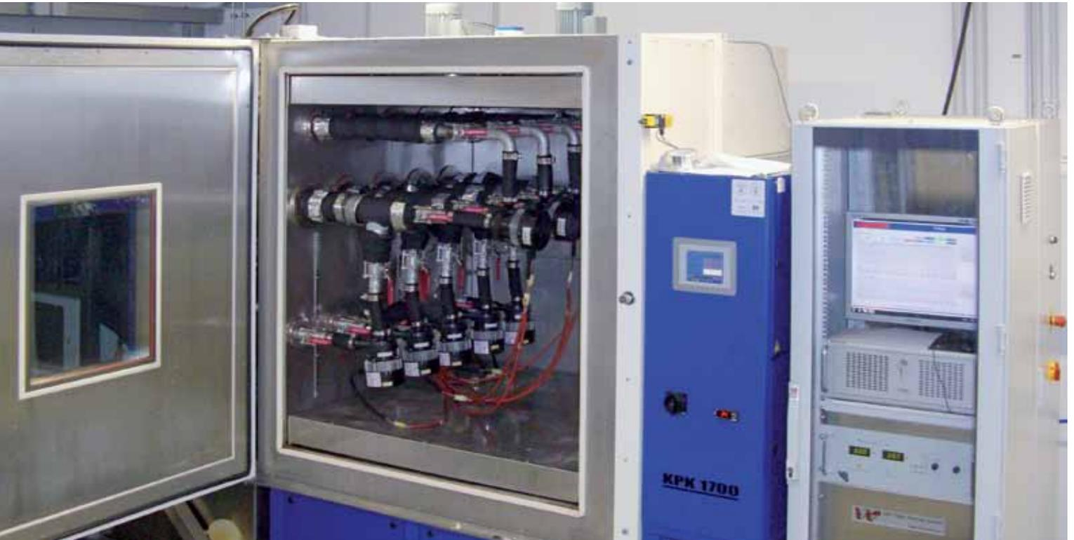
Arrangement of pumps on an endurance test stand.
