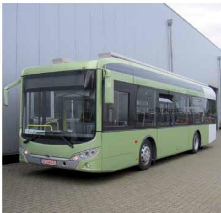
The Sileo electric bus from Bozankaya with the Citysphere air conditioning system.
