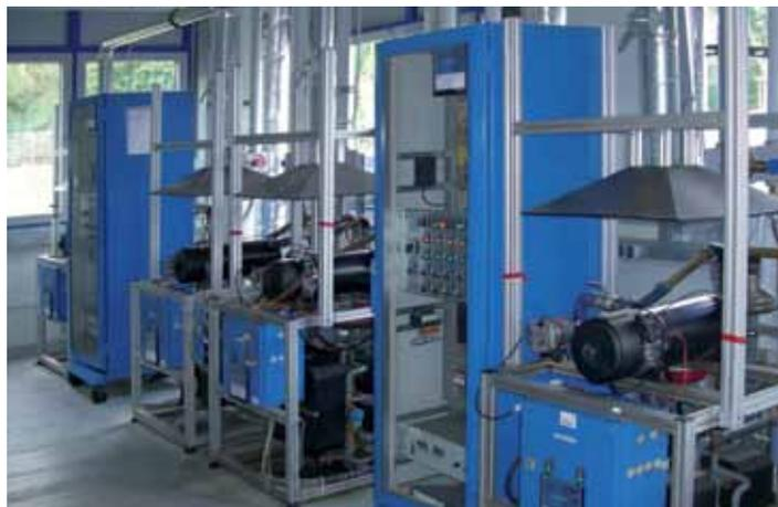
Thermo E heaters on the endurance testing stands at the Spheros facility in Neubrandenburg.
