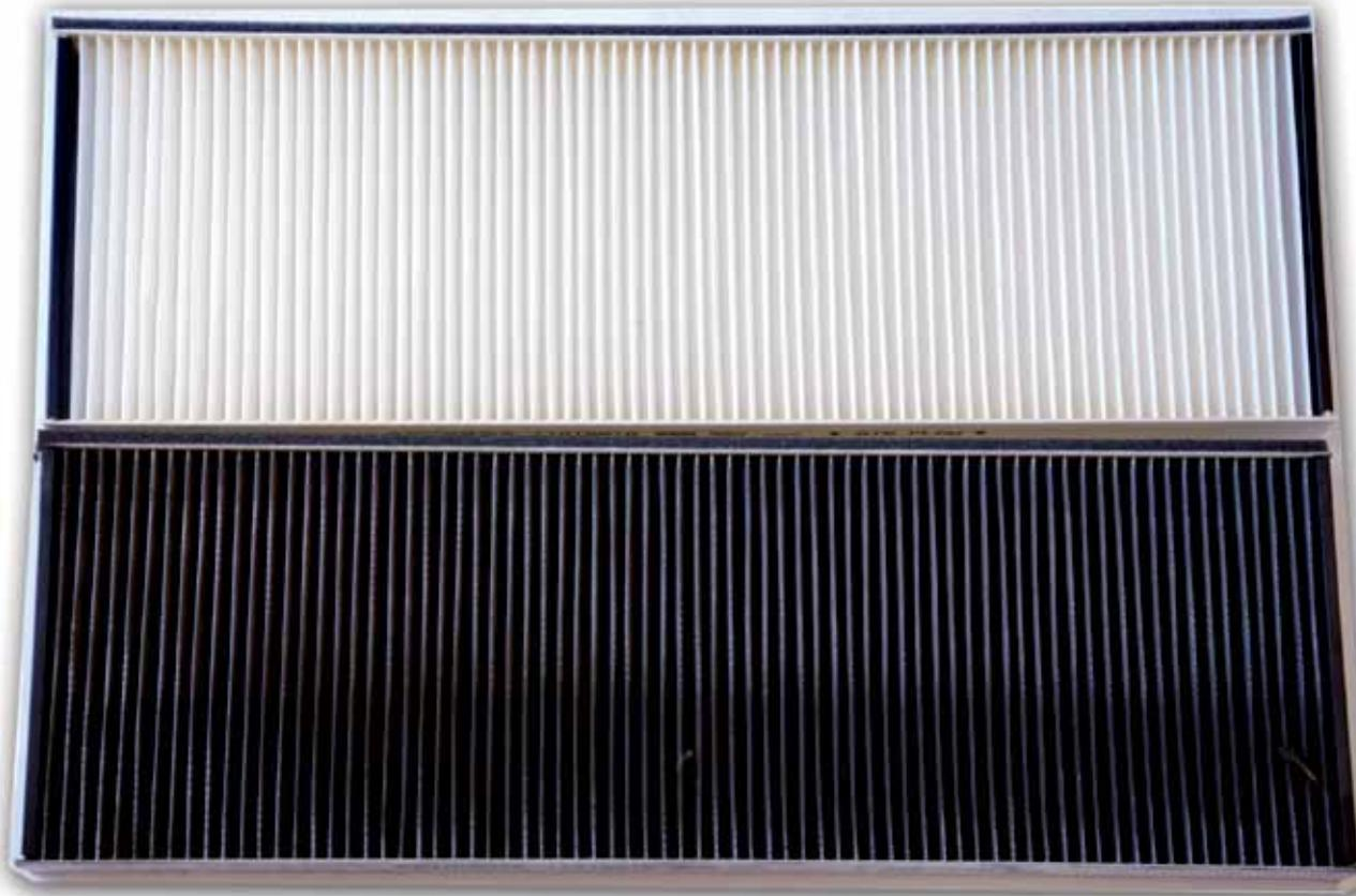
Comparison: New fresh air filter and filter after 3 months' use in normal road traffic conditions.
