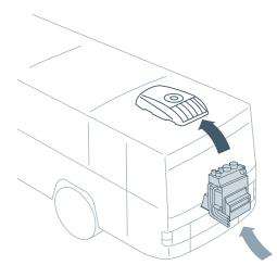
The condenser, located in the vehicle's standard heating ventilation unit, is connected to the rooftop unit by two refrigerant hoses. Air is circulated through air ducts at the driver's zone.
