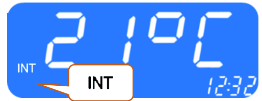
Figure 12 - SC1000 Current Room Temperature
